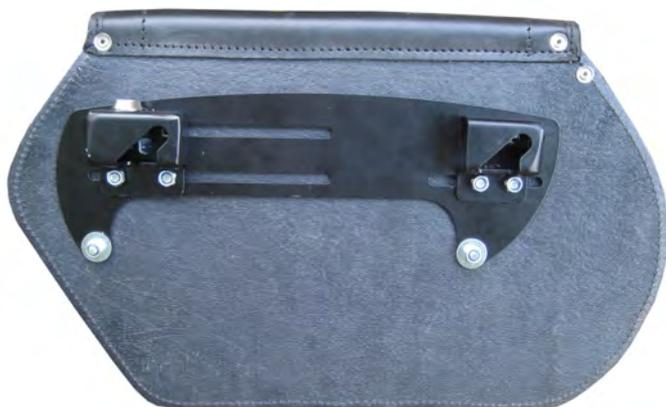
To mount the quick release system, 4 holes in the back of the bags have to be drilled.
